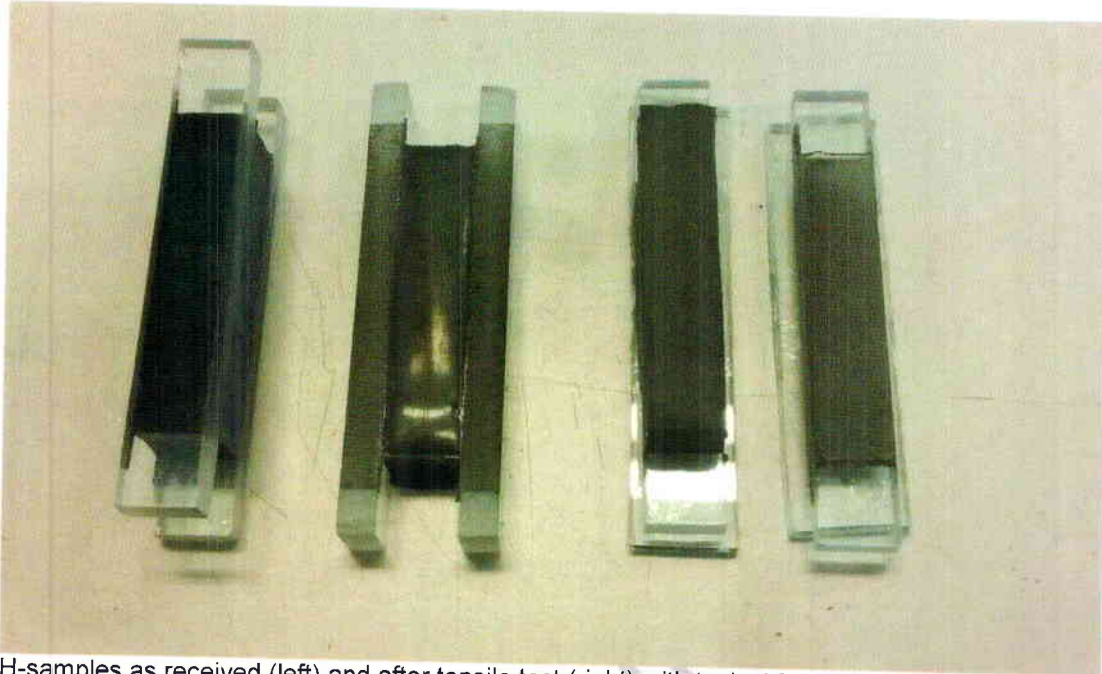
H-samples as received (left) and after tensile test (right) with typical failure type (cohesive)
